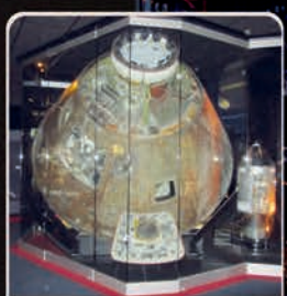
command module (CM): control centre & living quarters for crew
